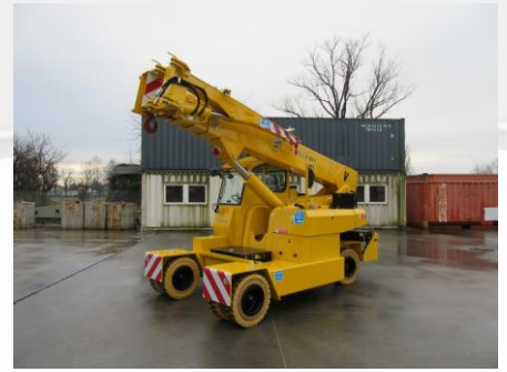
Hydraulic jib that can be turned on the boom side when not used
